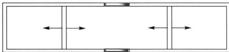
Figure 4.3. Schematic representation of the cell used for the determination of the equivalent resistance. 10 (Reprinted with permission from Elsevier Science).
